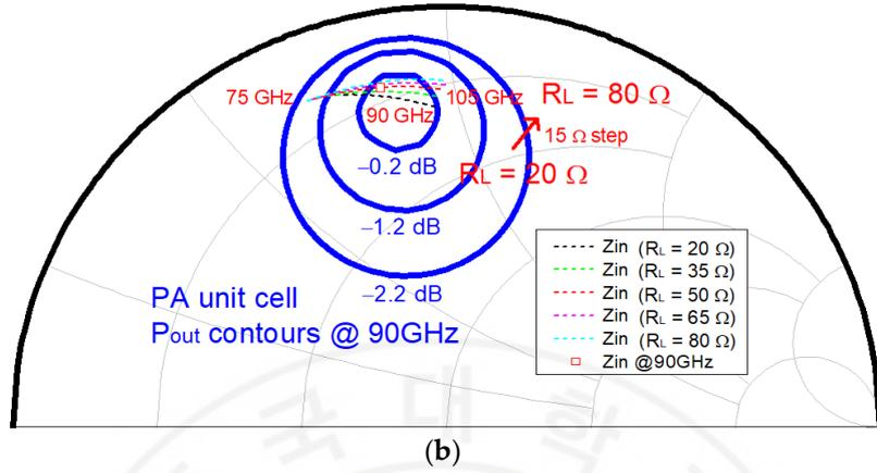
Figure 4.2-1 (a) Configuration of output matching network and (b) Power contours and the input impedance seen at each device with the load variations from 20 to 80  $\Omega$  at 90 GHz.
