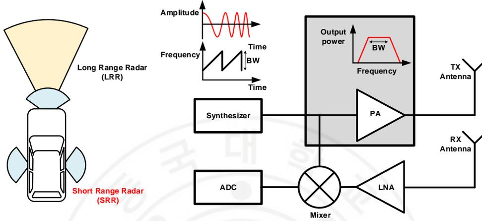
Figure 2.1-1 Architecture of FMCW radar
