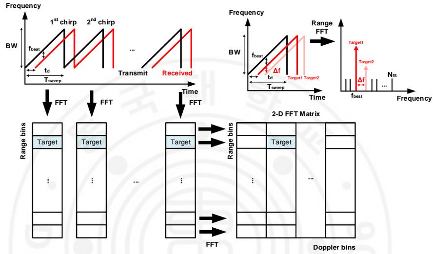
Fig 2.1-1 Range and doppler FFT for 2-D FFT matrix
