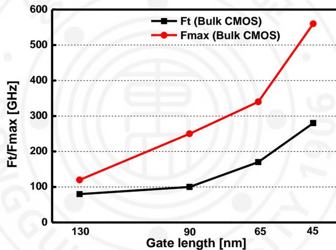
Figure 2.2-1 RF performance of bulk CMOS Technology
