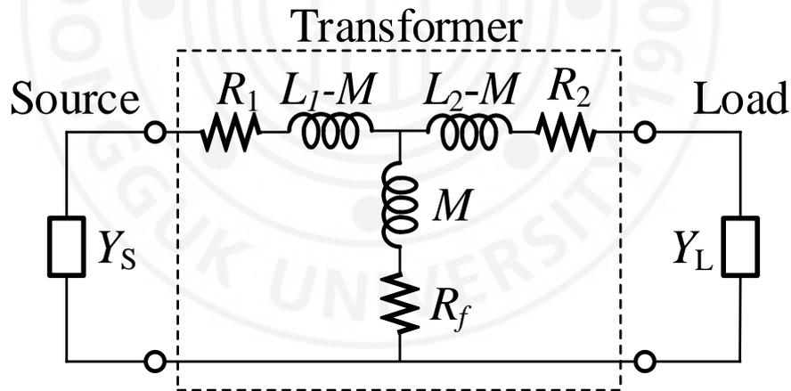
Figure 3.3-1 Six-parameter transformer model with general load and source
