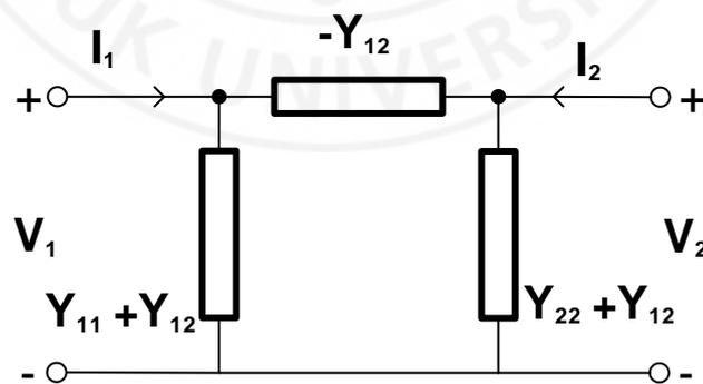
Figure 3.2-3 Equivalent circuit of Y-parameters
