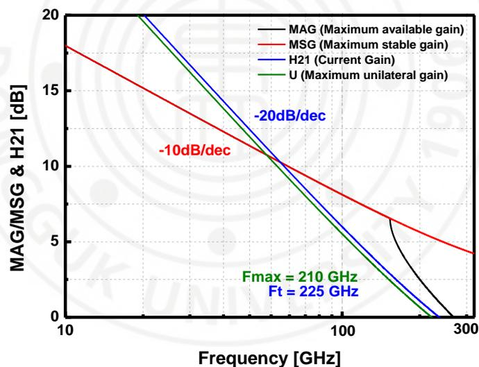
Figure 2.2-2 TSMC 65-nm CMOS device small-signal simulation results
