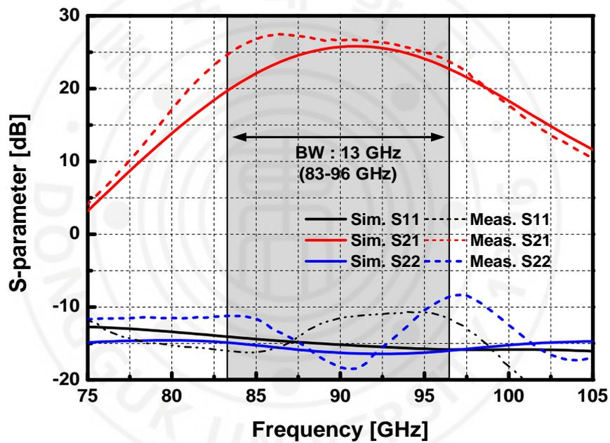
Figure 4.3-3 Measurement and simulation results of S-parameter of the W-band 8-way PA with a 50 Ω load.
