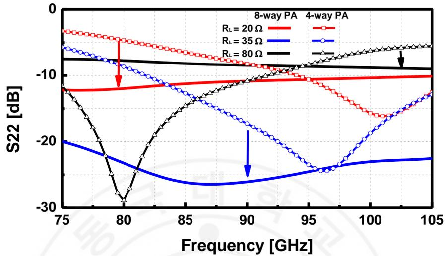
Figure 4.2-2 Simulation results of the output return loss of the 8-way PA (solid line) and 4-way PA (line with symbol) with the load variations.
