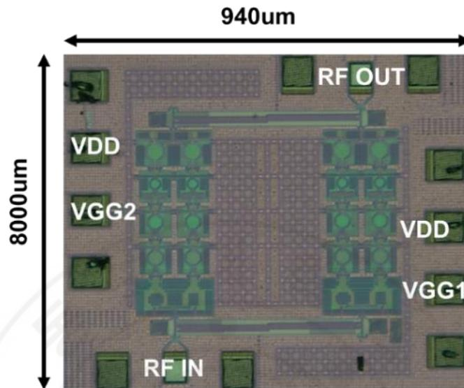
Figure 4.3-1 Chip photograph with the size of 0.94 mm × 0.8 mm including RF pads and DC pads.
