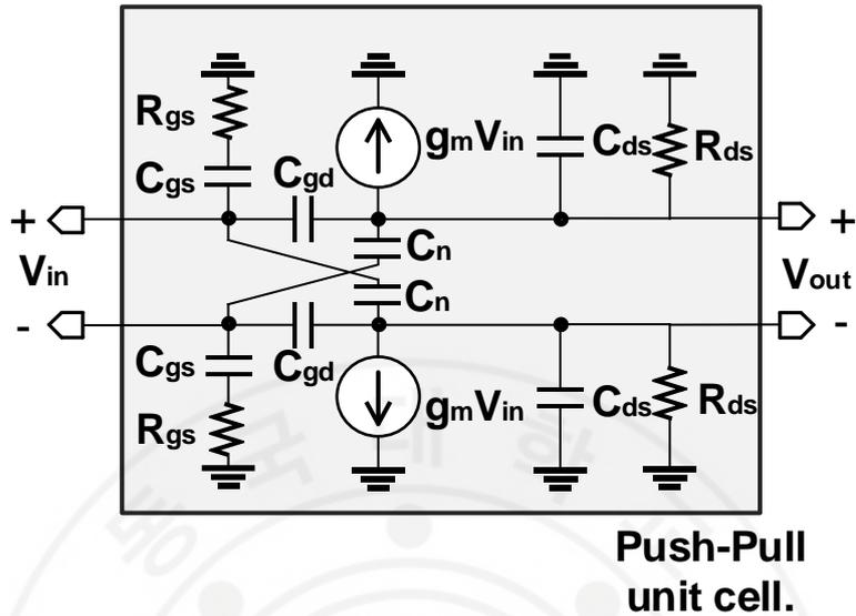
Figure 3.2-2 Small-signal schematic of differential common-source amplifiers with cross-coupled neutralization capacitors.
