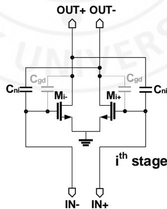
Figure 3.2-1 Schematic of the push-pull PA unit cell
