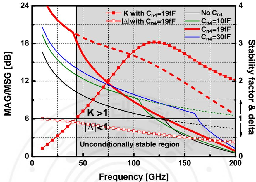
Figure 3.2-4 Simulated MSG (dashed lines)/MAG (solid lines) of the power stage differential pair depending on the neutralization capacitor  $C_{n4}$  and  $K$  and  $|\Delta|$  with  $C_{n4} = 19$  fF.
