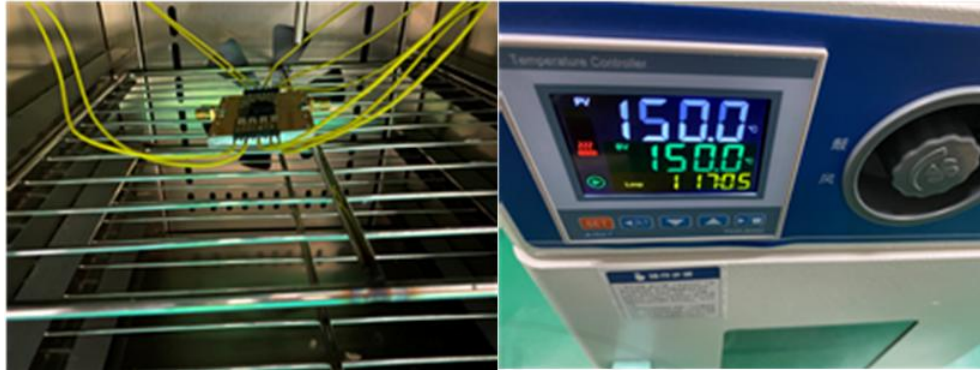
Figure 4.3-11 HTOL test setup
